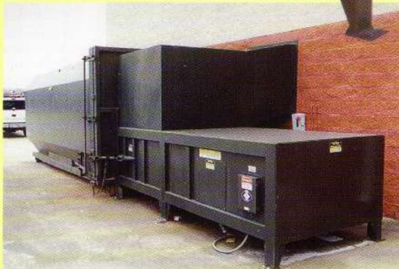
Photo shows 3 Yd. compactor and 40 Yd. receiver container with thru-the-wall installation.
